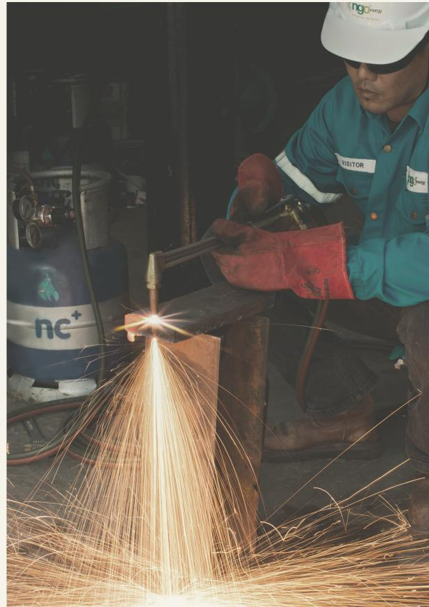
The nc+ metal cutting gas offers better quality of cut, increased safety compared to other cutting gases, user-friendliness as well as improved cost efficiency. This revolutionary alternative cutting gas solution is exclusively offered by NGC Energy.
